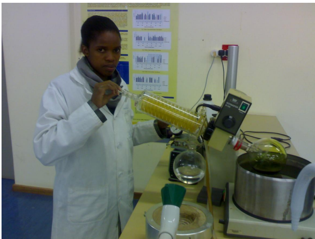
Extraction process of L. javanica using a Rotavapor system.
