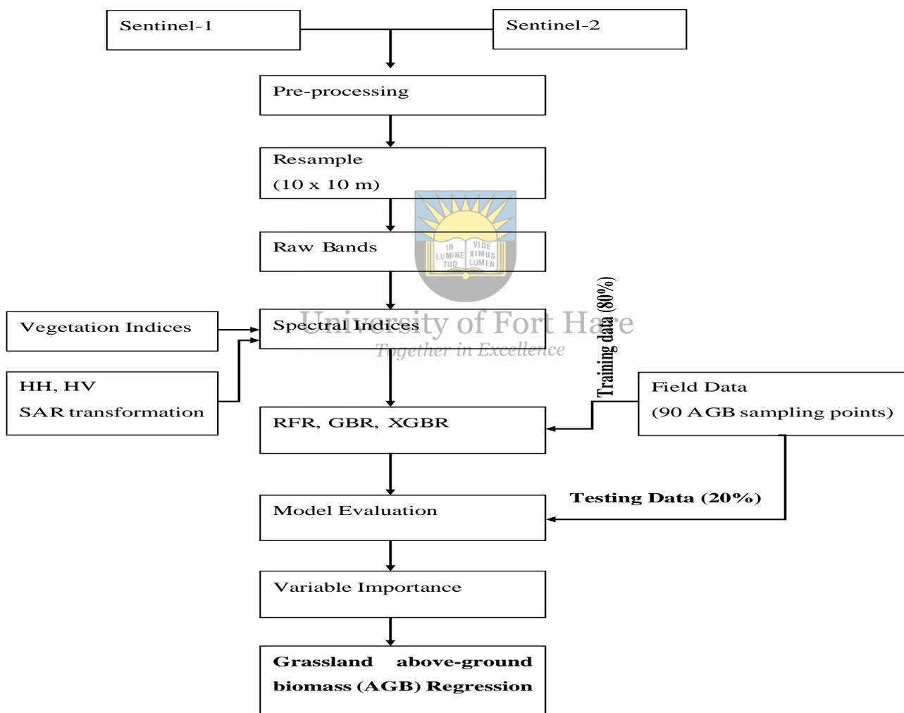
**Figure 11:** Flowchart of satellite –image processing and generation of AGB models on ML techniques
