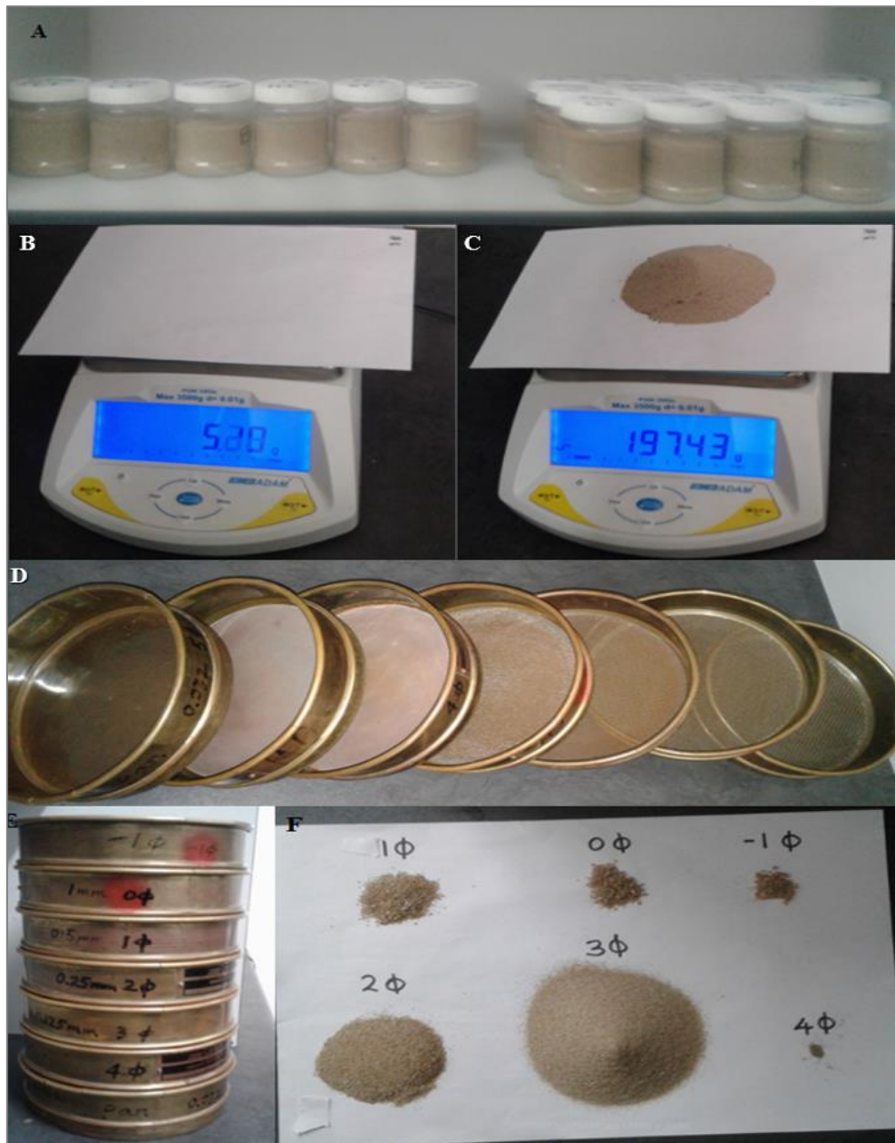
Fig.3.3: The process and equipment for the grain size analysis.
