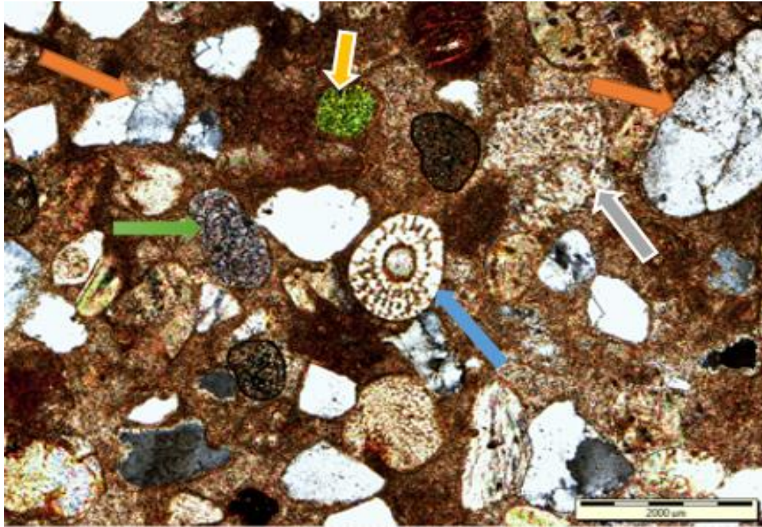
Fig. 5.9: Photomicrographs of various sand grains showing quartzite lithic (orange arrows), siltstone lithic (green arrow), glauconite (yellow arrow), plagioclase (grey arrow, partially replaced), foraminifera (blue arrow) and various other grains, sample 32 from Swartkops estuary.
