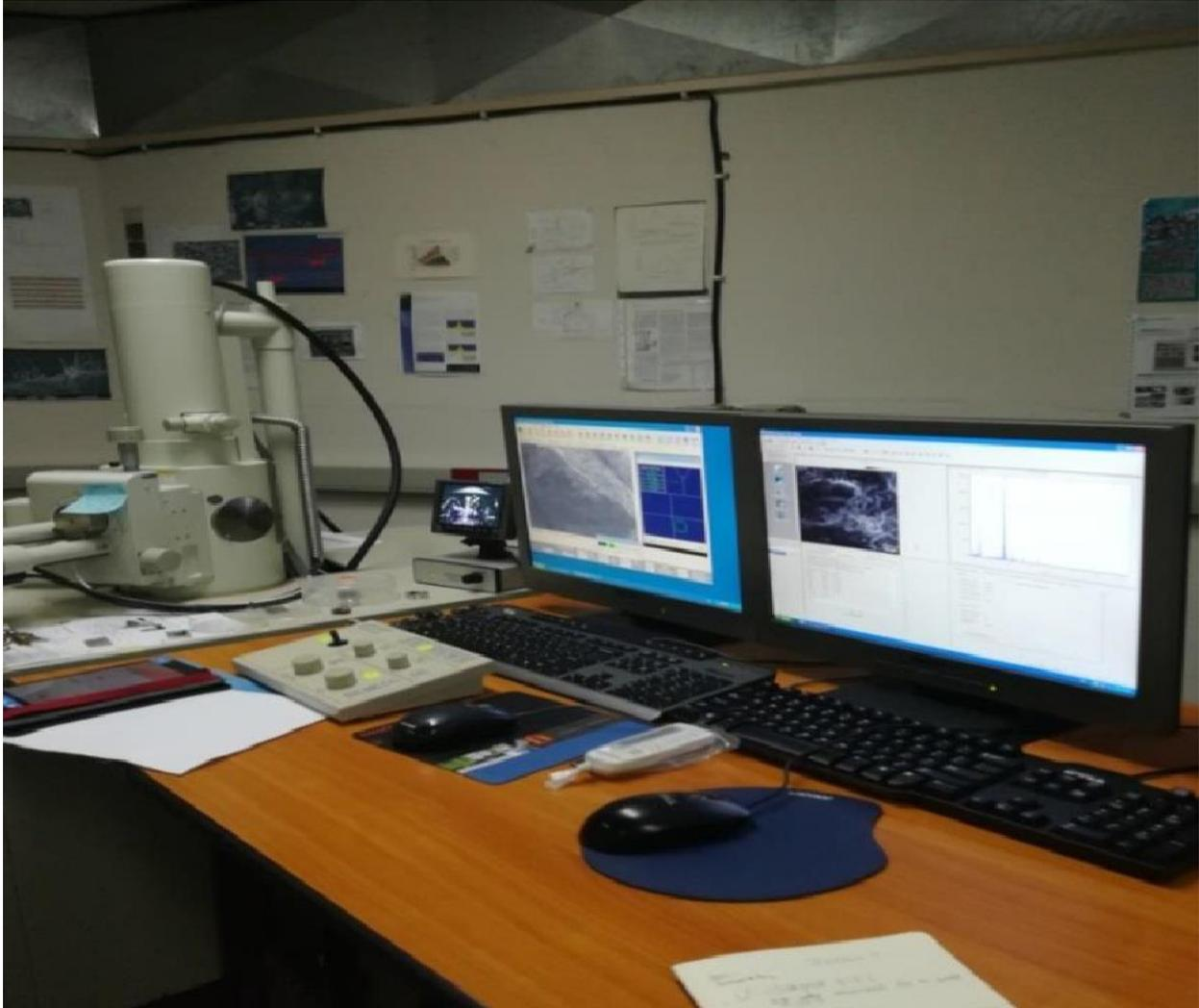
Figure 3.7: JEOL JSM-6390 LV model of Scanning Electron Microscope.
